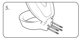
Insert the M10 Bolts through the Orbis fixing holes.
