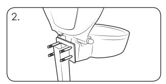
Insert the Orbis with the bolts through the holes of the Orbis Post.
