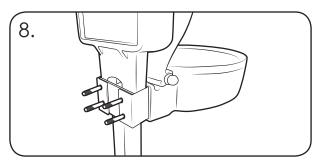
Locate Orbis with fixing bolts in to the 2 Point Bracket, Orbis Post and Sign Carrier.
