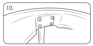
Secure in position with M10 Washers and Nuts using 17mm Spanner and 8mm Allen Key.
