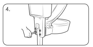
Secure in position with M10 Washers and Nuts using 10mm Spanner and 8mm Allen Key.
