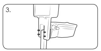
Locate the Sign Carrier's fixing holes on to the exposed bolts protruding through the rear of the Orbis Post.
