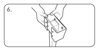
Align the 2 Point Bracket with the fixing holes on the Orbis Post.
