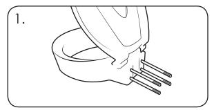
Insert the M10 Bolts through the Orbis fixing holes.
